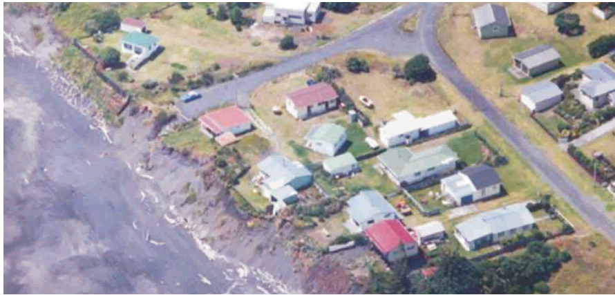
Figure 7: Mokau spit - properties and dwellings threatened by erosion in mid 1990s as a result of significant fluctuations of the shoreline near the Mokau River entrance. (Photo: J Dahm).
