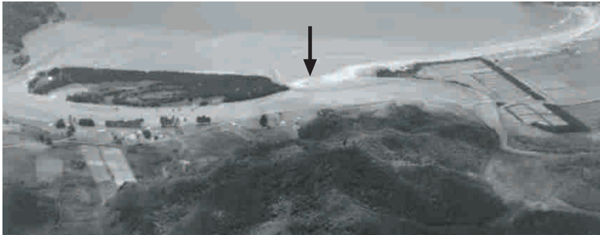
Figure 4: Example of spit breach. Aerial view of Kennedy Bay sand spit taken in 1982 – showing a second entrance (arrow) formed by a spit breach. The normal entrance is further north (far left of photo). The breach was eventually closed by human action. Left to natural processes, the second entrance may have gradually migrated northwards eroding the forested land between or it may have closed naturally.
