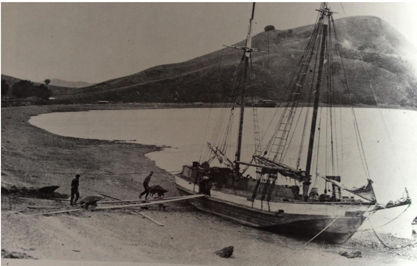
Thistle loading shingle at Pahiki Island. With a short wheel and a good bank of shingle they are loading two planks simultaneously — not a common practice. Note how the scow's bow is down the beach to give a downhill run when the barrow hits the deck.
