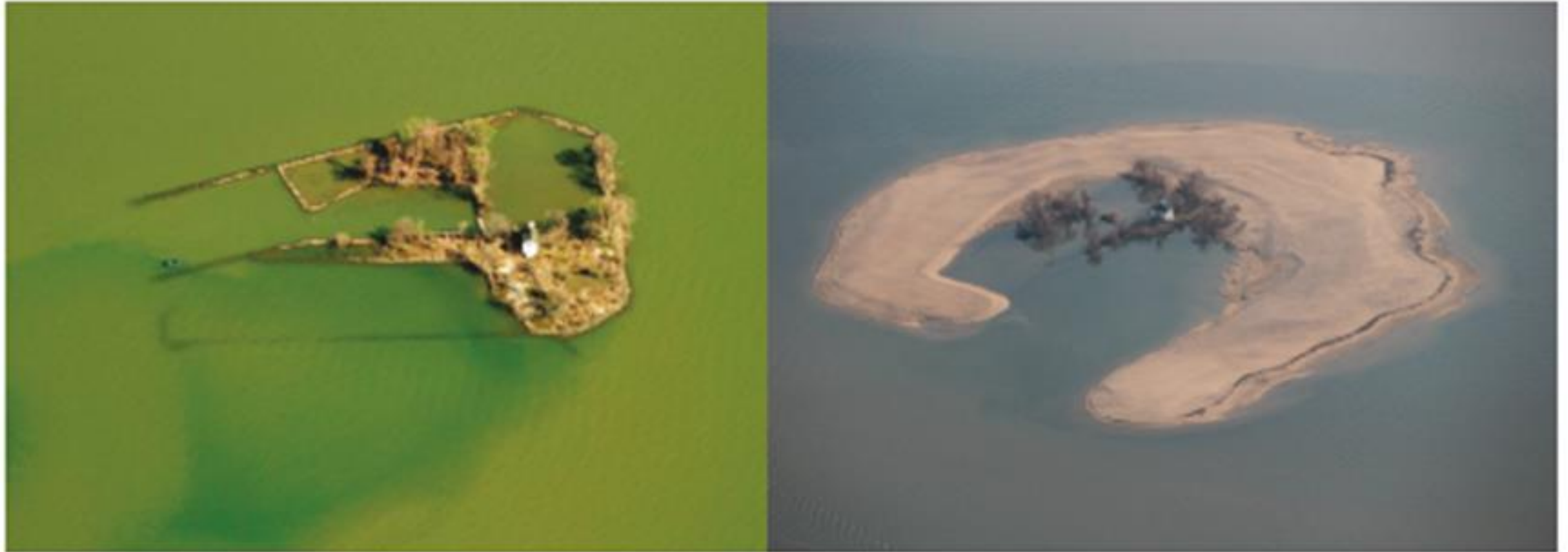
Figure 7. Battery Island before (left; 2011) and after (right; 2013) unconfined placement of dredge material
