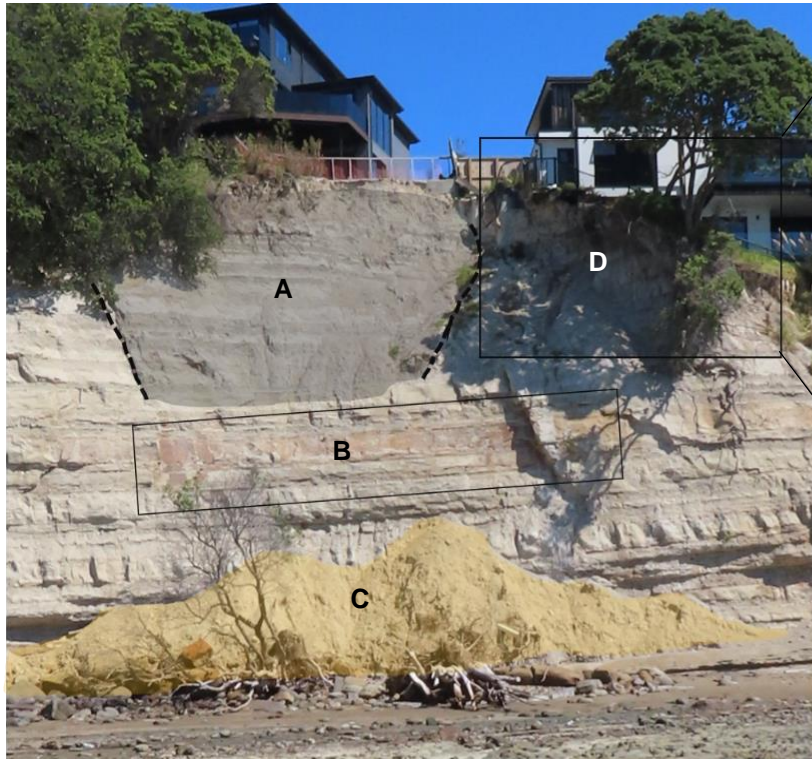
A) Location of the wedge failure with its associated vertical jointed surface/failure plane (black dashed lines). B) Failure of sandstone bedding plane C) Talus formed due to the accumulation of the debris supplied by the two failures above. D) Collapse of weathered soil at the cliff top has exposed the Pōhutukawa tree root system and foundations of the properties. A properties' deck can be seen hanging mid-air.
